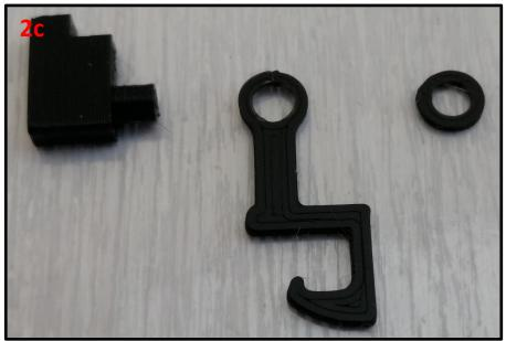
2d – Take the coupler hook and push it onto the round extrude of the coupler holder as in the picture below.
