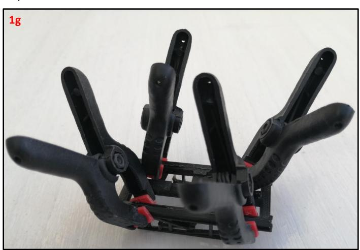
IMPORTANT! PLA Plastic will deform and melt like any other plastic if left on a hot/near a surface such as a radiator. Leave your parts to dry in a warm ventilated area, or at room temperature. It is also strongly advised that you do not leave parts to dry in a conservatory as the magnification of light can also cause the PLA plastic to deform.
