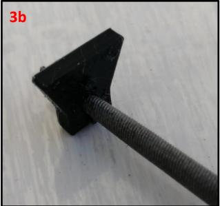
**3b** – Remove any extra plastic or strings from the pieces with any of the following tools and equipment listed on **page 3**. You may also want to use a small round file to remove any debris in the wheels holders, see above.
