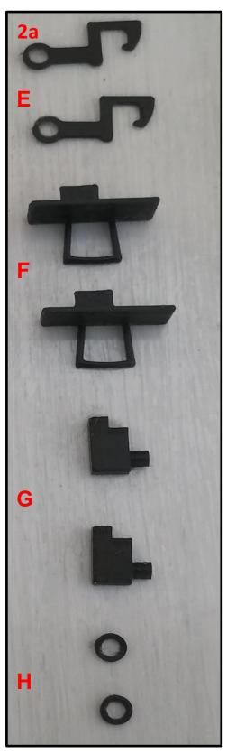
**2b** – Remove any extra plastic or strings from the edges of the pieces with any of the following tools and equipment listed on page 3.
