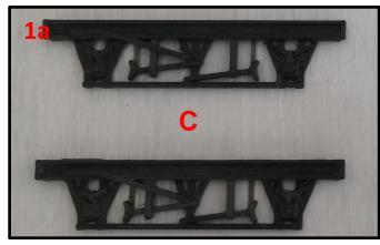
**1b** – Remove any extra plastic or strings from the edges of the pieces with any of the following tools and equipment listed on **page 3**.
