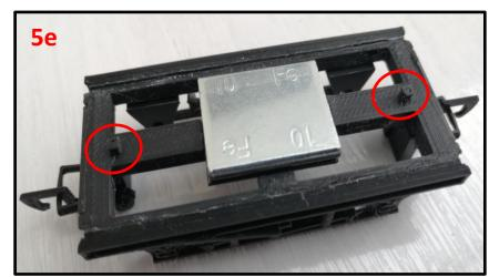
**5f** – Place glue around the two small extrudes on the chassis/base. Aim not to apply to much as when you push the wagon body down it may squirt out.
