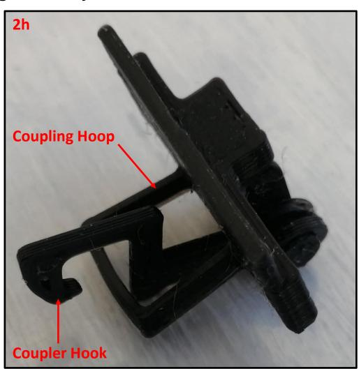
2i – Also check that the edges of the upside down letter "L" on the coupler hoop are flat and smooth. If they are not use a flat file to smooth the edges down.
