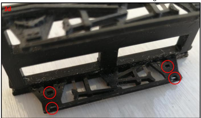
**3e** – Place a small amount of glue into the holes and the area between them. Take a wheel holder and push it into place. Make sure it is aligned as shown in the picture below and apply pressure until it holds in place.
