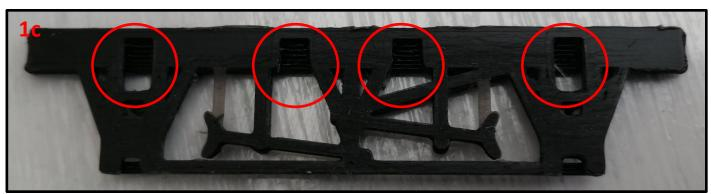
1c – Notice how the back of the chassis has 4 slots missing, see above. This is to allow it to attach to the sides of the base.
