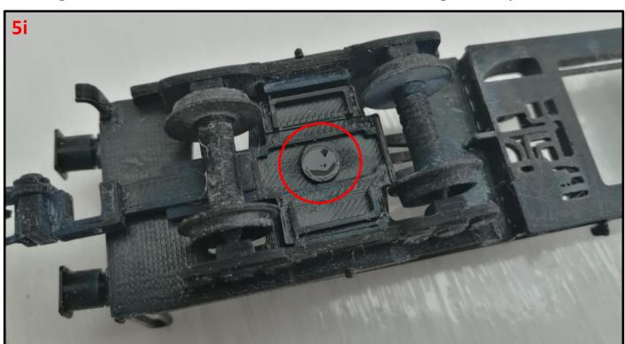
**5j** – The 5g weight will clip over the bogie holding ring onto the brackets. First test that the weight will clip into the brackets.
