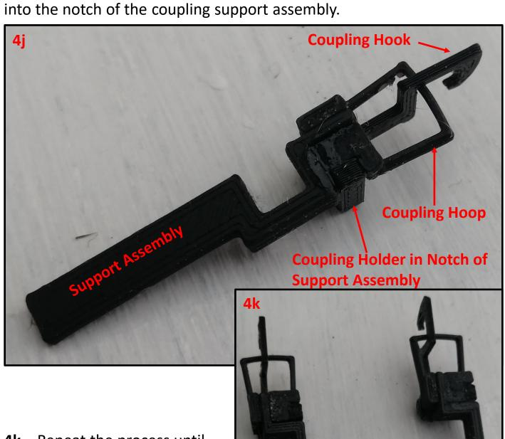
**4k** – Repeat the process until you have two fully assembled couplings. Please ensure no glue gets on moving parts, the coupling hook must be able swing and move freely. Leave to dry and move onto the next step.
