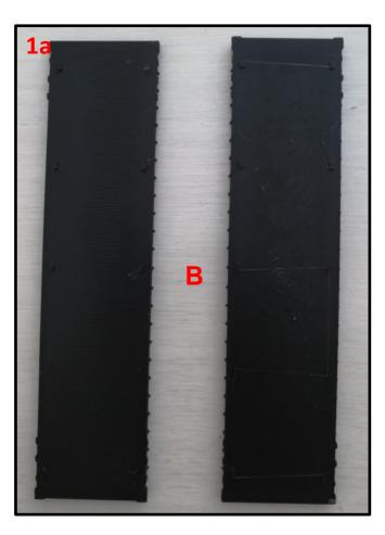
**1b** – Remove any extra plastic or strings from the edges of the pieces with any of the following tools and equipment listed on page 3.
