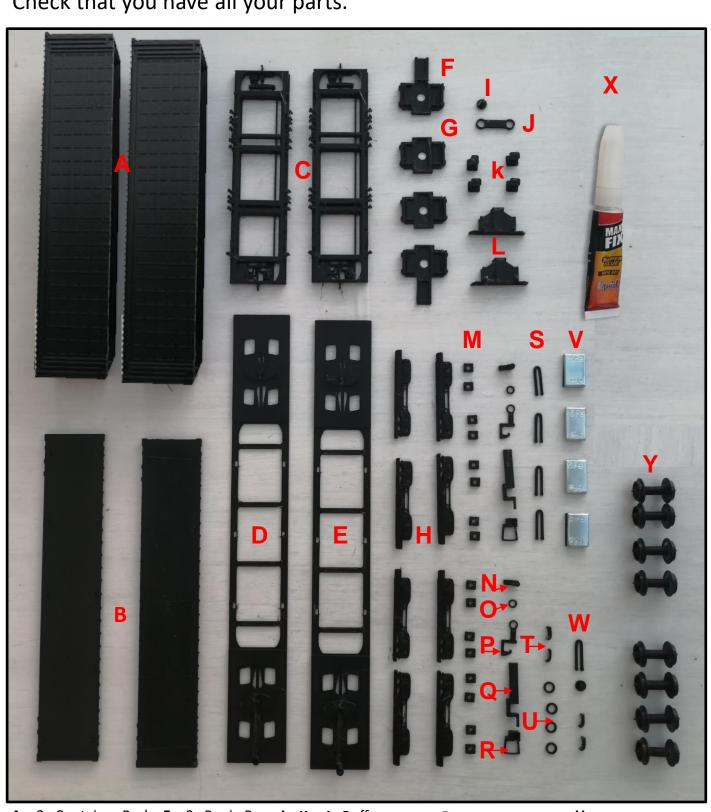
A - 2x Container Body F - 2x Bogie Base A K - 4x Buffers
