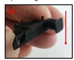
**2j** – Repeat this process until you have attached all 4 buffers to the base tops. Leave both pieces to dry at room temperature.
