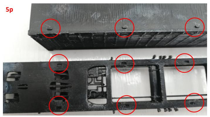
**5r** – To clip the Container into Place flip both pieces onto their sides and align the Extrudes and the Square Holes.
