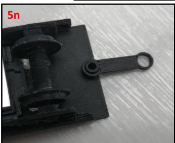
**5o** – Take the coupling pin and place it into the hole. Now with force push and clip the pin into place. Ensure you push vertically down as not doing so could cause the pin to break. You will not need any glue to hold this down. The base Coupler Should swing freely.
