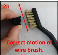
**2h** – Remove any extra plastic or strings from the pieces with any of the following tools and equipment listed on **page 3**. For **Part L; Base Tops** it is important that if any brush is used, it is used in an up and down motion along its top surface, see picture above.
